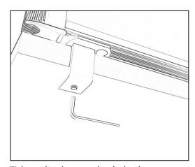
Tighten the clamp to the desk edge using an allen key to secure the screen in place.
