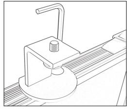
2) Position the bracket on top of the sliding plate where desired and tighten using a bolt and an allen key.
